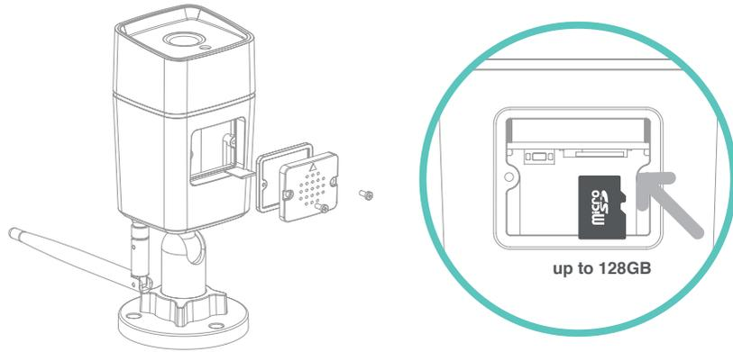
**UK** Before installation insert a compatible microSD card, class 10 up to 128GB (not included). Remove the two screws that secure the bottom panel and insert microSD card into the slot. Secure the bottom panel in place with the two screws.
