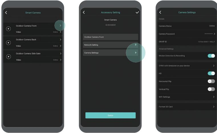
**UK** Change camera password / Motion detection & recording / Sync timezone / Record in HD or SD / Horizontal and vertical flip / Update wi-fi settings / Format SD card.
