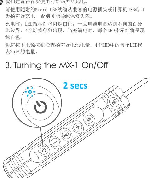
To turn on the speaker, press and hold the power button for approximately two seconds; a blue power indicator light will appear and the speaker 'On' tone will sound. If the speaker has previously been paired to a device, they will reconnect automatically.
